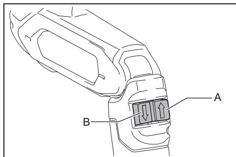
To start the tool, simply push the switch on the A side for the clockwise rotation and the B side for the counter-clockwise rotation. Release the switch to stop.
