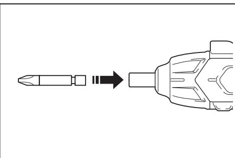
To install a driver bit, push it firmly into the driver bit holder. To remove the driver bit, pull it out of the driver bit holder.
