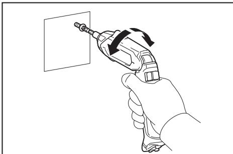
Switch off the tool, and then turn the tool.
