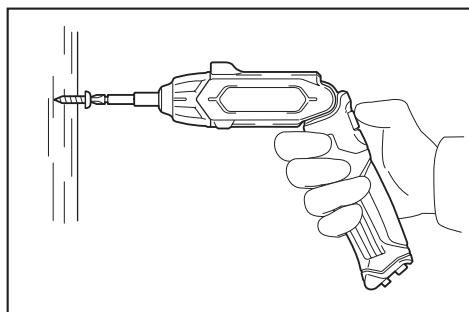
Place the point of the driver bit in the screw head and apply pressure to the tool. Then switch the tool on. When the screw head and surface of the workpiece becomes flat, release the switch.
