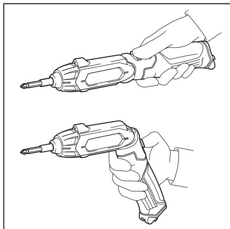
The tool can be used in two ways; a straight shape and a pistol shape which are selectable according to the conditions of workplace and screwdriving.
